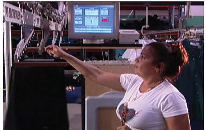
An RF-driven system eliminates the need for a third sort. A significant benefit is that the garments are in route-delivery sequence on the second sort with only one handling.
