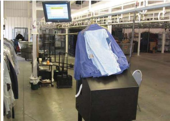
**Clean Garment Bundle Reader** – There's no longer a need to scan or count individual clean pieces to obtain a bundled-garment count. With multiple-read chips, you can now read all the chips in a hanged bundle, and verify the contents electronically, prior to staging it in the route-ready area. Productivity is in the 3,000+-piece per-hour range.
