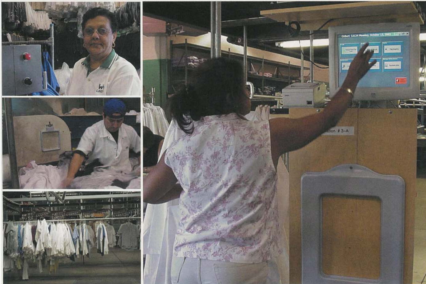
RFID technology can be found throughout the W.H. Linen plant, including inventory (top left) the soil room (center left) route make-up (bottom left) and sorting (above right).
