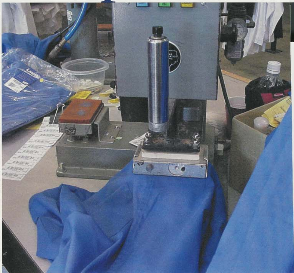
RFID chips are heat sealed with a bar code on items entered into inventory.
