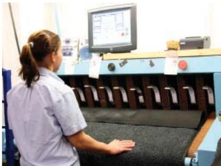
LEFT: Thanks to Positek's RFID enhancement, the usual multi-step procedure of loading out mats is reduced to two: rolling and route-building.
